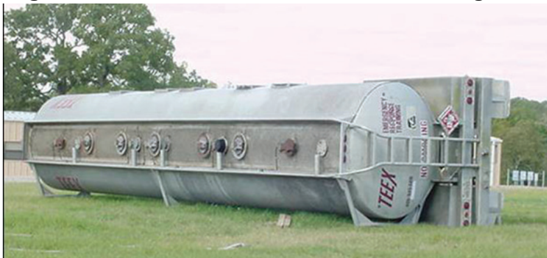
Figure 3.2: Overturned MC-306/DOT-406 Cargo Tank
